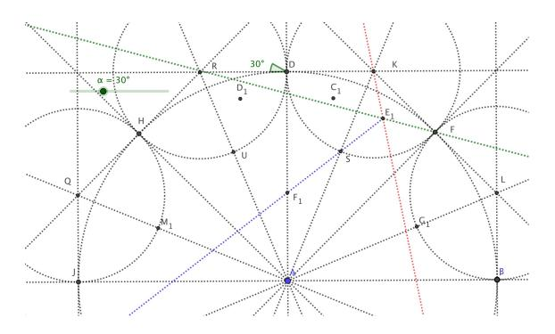
Now we can connect  $DC_1SF_1UD_1$  to form the top petal. In addition note that the segment  $SF_1$  and  $UF_1$  are extended to the next radial lines. This will be helpful in forming the inside of the rosette.
