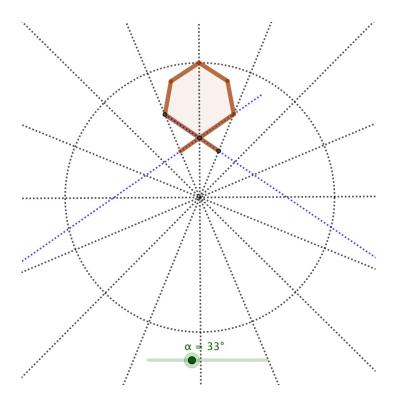
Now repeat this procedure around each of the 8 vertices of the original octagon to achieve the following. Note these typical convergent rosettes below are formed from an incident line obtained by connecting intersections of the original circle with various radii, thus not requiring the use of a protractor measure out a specific angle.
