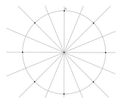
Then connect the 8 points shown to form an octagon and construct tangent lines at these 8 vertices as shown.
