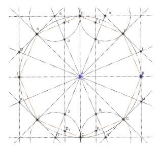
Now repeat this same process three more times to create 3 more sets of parallel lines. This is done using circles at Q,P,M,L then K,L,O,P and then Q,R,M,N. Each of these sets of parallel lines intersects the octagon at points that are vertices of the petals. The picture below removes the diameters and tangent lines to better illustrate these sets of parallel lines.
