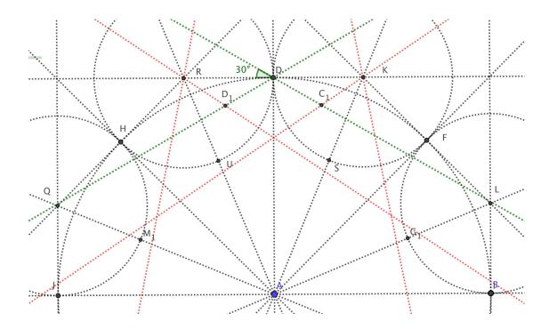
All that remains to be identified is the lower point of the petal. To find this we repeat the steps above about point F, by constructing a line at 30 to the tangent at F and by bisecting FKS. These two lines intersect at  $E_1$ .  $E_1$  is a vertex of the next petal but is also needed to locate the bottom of the first petal as shown. Extending  $E_1S$  to the vertical diameter of the original circle identifies  $F_1$  which is our remaining point.
